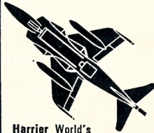
Harrier World's first V/STOL combat aircraft; can operate from a 50 ft. farmyard or jungle clearing.
